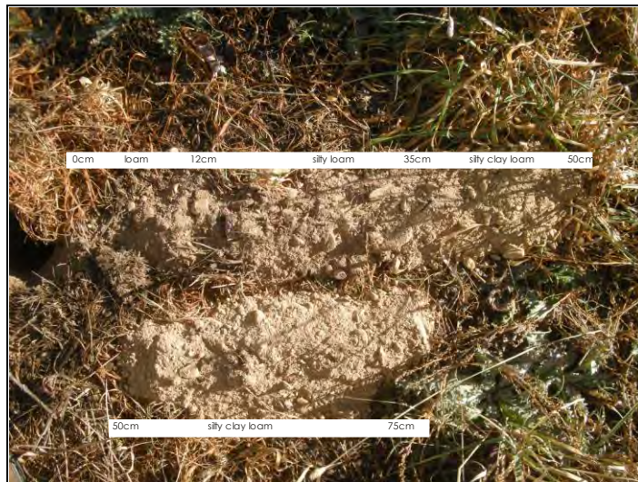
Photo 2: moderately deep yellow dermosol found on the areas mapped as hillslope (profiles 3 and 4). These soils have a weakly structured silty loam upper layer grading to clay loam subsoil and extending to a depth of 70-90cm.
